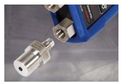
Crystal Pressure Fittings<sup>•</sup> are machined in high-strength 316 Stainless Steel to operate at 10000 psi/700 bar. Removable CPF adapters shift everyday thread wear away from the HPC40 Series' ports, while a self-venting weep hole alerts you before you disconnect from a pressurized system.
