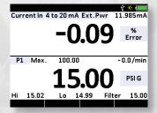
mA loop span. For example, if you are testing a 30 psi full scale pressure transmitter with a corresponding 4-20 mA signal, you can program into the calibrator a 0 to 30
